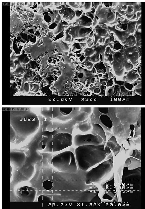
**Figure 3.** Characterization of hydrogels. SEM images confirmed that chitosan hydrogels containing Se NPs are porous structures with suitable pore sizes for cell penetration, migration, and attachment.
